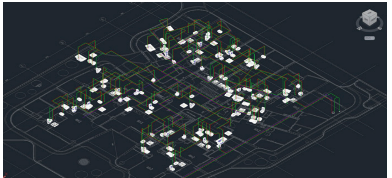
A 3D floor plan directly takes into account all real pipe lengths and thus ensures maximum planning accuracy.
